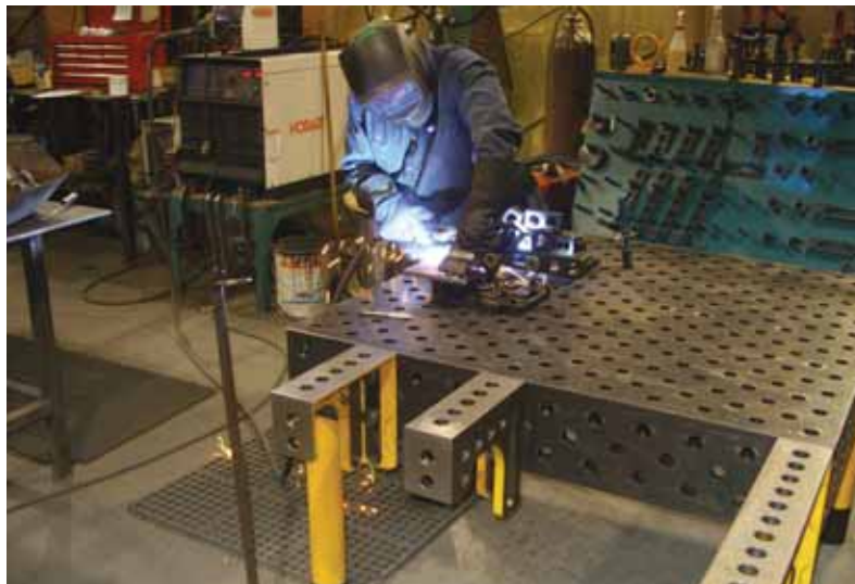
The modular fixturing system shown here has provided various benefits at John G. Wilson including improvements in productivity.
